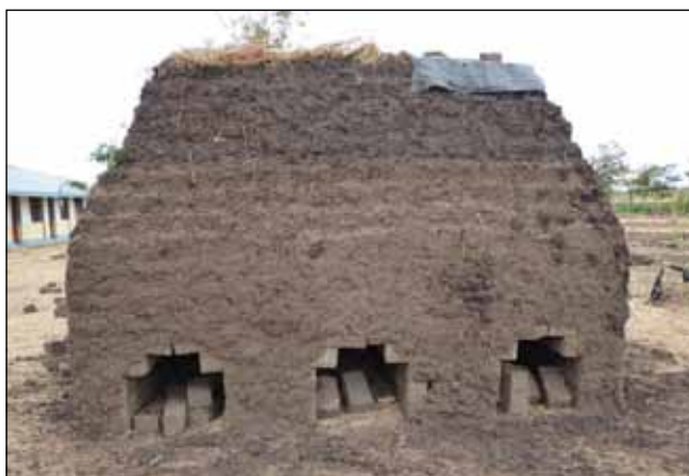
Figure 4.6: A Commonly Used System of Burning Bricks which use Huge Amount of Fuel Wood
